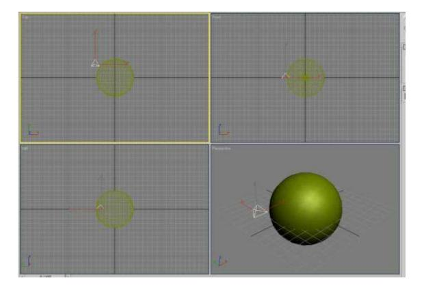
Now, we need to bind the bomb to the sphere. So click on the "Bind to Space Warp" tool (highlighted in yellow). Click on the bomb and drag your mouse to the sphere. The sphere will flash white for a second. I have dragged the time slider (at the bottom of the screen) to frame 12 to see the effect.
